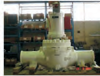
22" ANSI 1500# Hydraulically Operated Subsea SSIV
